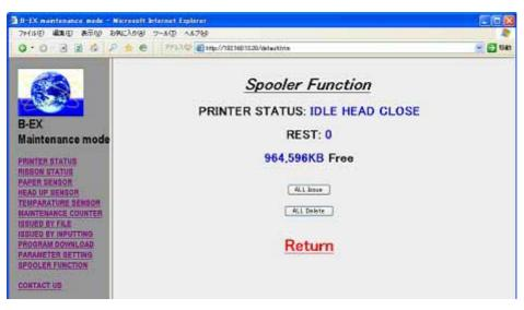
"PRINTER STATUS:" indicates the current printer status, "REST:" indicates the remaining print data count, and "\*\*,\*\*\*KB Free" indicates the available space in the printer.
