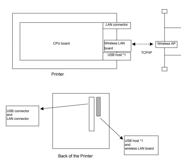
\*1: The USB host is used in the functions of the Web printer, e-mail transmission/reception and FTP when the use of external memory is specified for the Web printer function.
